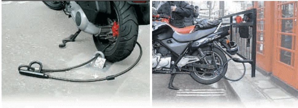
Figure 26: Example of Ground Level/Raised Locking System
