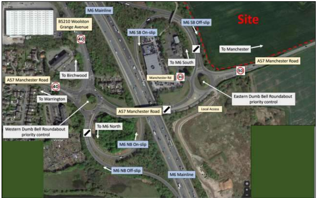
Figure 2.6: Plan View of M6 Junction 21 Woolston Interchange
