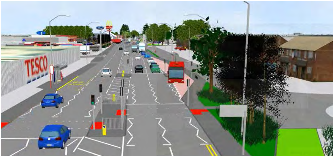
Figure 25: Pre-signals upstream from the Tesco Junction allowing Bus Priority (traffic model).
